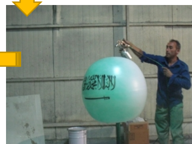
Apply Conventional Green C. Paint.
